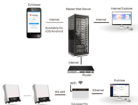
Figure 6.1-1 Wi-Fi EzLogger Pro Monitoring System Diagram
