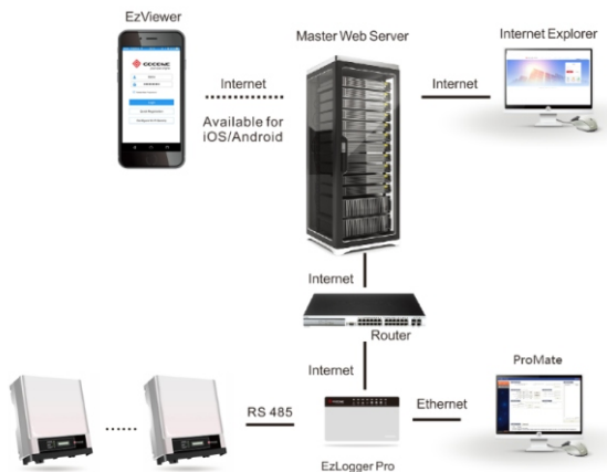
Figure 5.1-1 LAN EzLogger Pro Monitoring System Diagram
